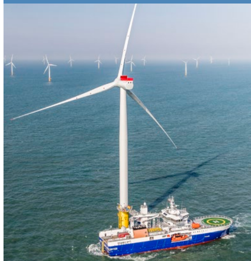
The Bibby WaveMaster 1, a Damen ASV 9020. Good seakeeping behaviour was an essential design goal for this vessel, which provides a comfortable working environment for offshore personnel.
